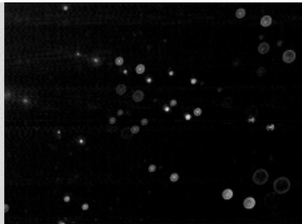
Figure 3 – Double-pulse TV data (M: 1.2, particles: 5 µm polystyrene)
