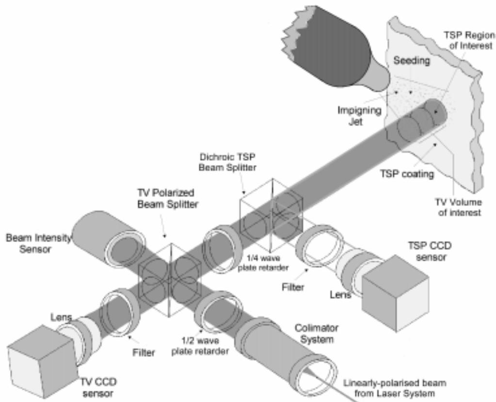
Figure 1 – Tunnelling Velocimetry (TV) schematic system diagram.
